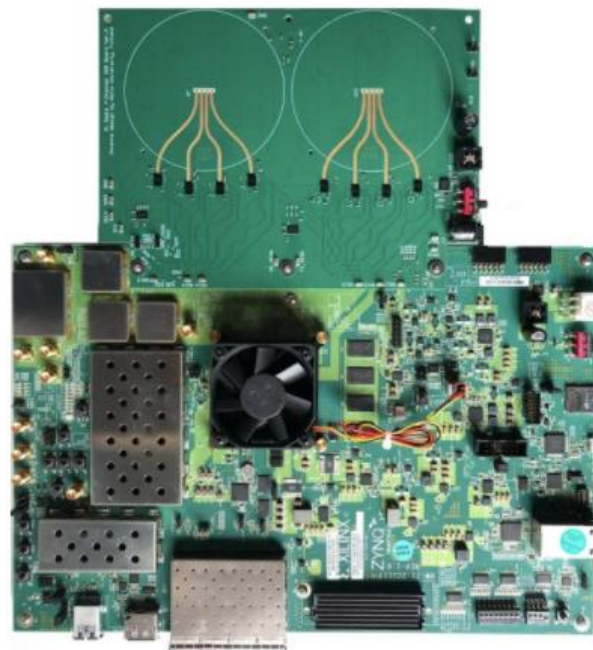
Fig. 11. Pi Radio 60 GHz array SDR for 6G experimentation, consisting of 4 transmit antennas, 4 receive antennas, and Xilinx ZCU-111 RF SoC compute platform for SDR and ML applications.
